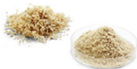
Optimal preparation of a wood sample with the cutting rotor
