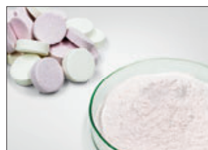
Cookies and vitamin tablets before and after comminution in the Knife Mill PULVERISETTE 11
