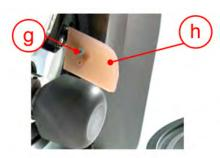
The fastener (g) of the scraper should not be tightened too firmly so that the scraper can be moved around the Philips screw (g).
