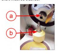
Inserting the pestle shaft into the bearing locks the pestle into its working position again. When inserting the pestle shaft, make sure that one of the milled spanner flats (b) on the pestle is located next to the drive screw (a).
