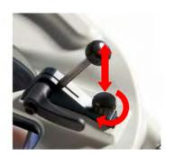
7. Turn the screw to the right to reduce the contact pressure of the scraper against the mortar so that the scraper lightly touches the wall.
