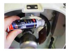
Apply the lubricant sparsely to the contact surface!
