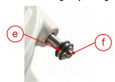
It is positioned radially in relation to the main rotation of the mortar. The desired contact pressure is built up by turning the adjusting screw (e). To do so, turn the screw (e) to the right until the display cylinder is visible (f). The contact pressure can be read on the display cylinder (f). For most applications, the lateral contact pressure is set so that the 1st ring or the 2nd ring is visible.
