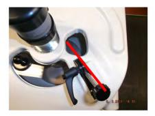
Tilt the guide rod while turning the scraper to the left to align it with the guide rod.
