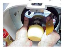
The pestle is held in place with a catch holder and can be easily removed without tools.
