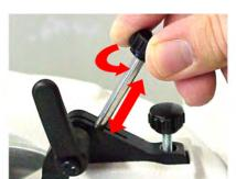
Move the scraper against the wall and onto the bottom of the mortar by turning it to the left.
