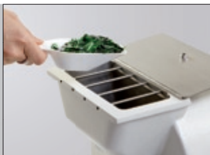
Filling of the funnel with pre-crushed glass bottles
