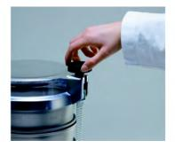
By turning the knurled knobs to the right, tighten the sieve stack evenly until the toothed belts are tightly clamped!
