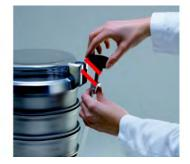
10. Then attach the knurled knobs to the holders of the sieve cover!
