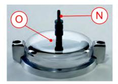
At the quick-release coupling (N) on the plexiglas clamping lid with 2 rotation nozzles, connect a hose (with hose clamp), through which the rinsing liquid can be fed. Feed just enough water or alcohol (only possible with additional pump) to prevent a backup in the sieve set.
