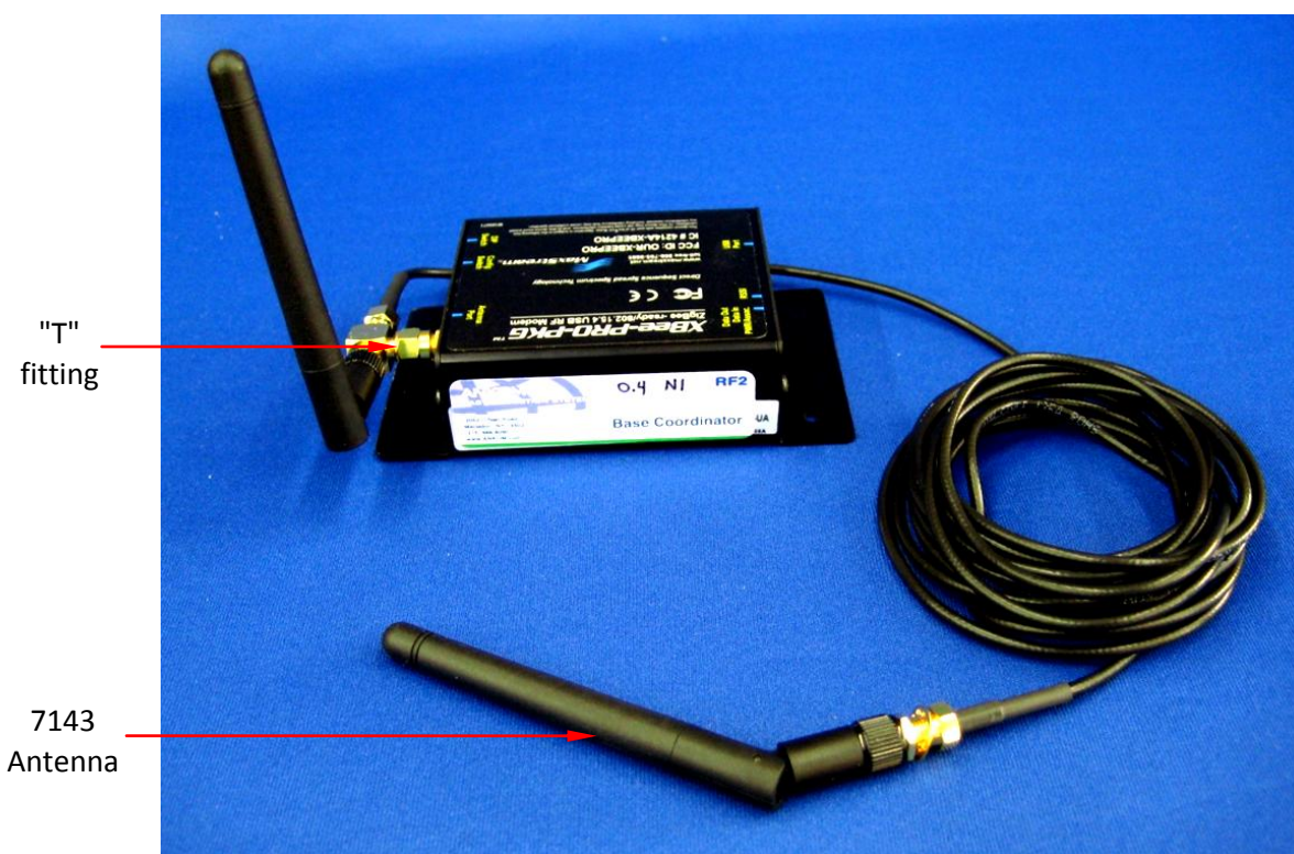
Antenna Extension Assembly (part # RF29) connected to the Base Coordinator
