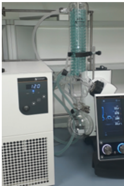
Fig. 4: Rotary evaporator system with recirculating chiller
