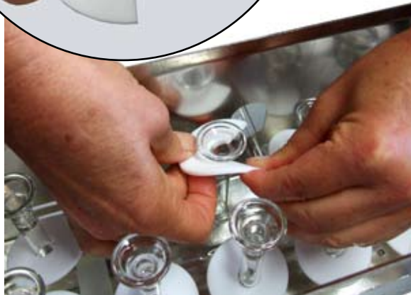
Bend the PTFE plates in order to take them out (and bend them back in form afterwards!)
