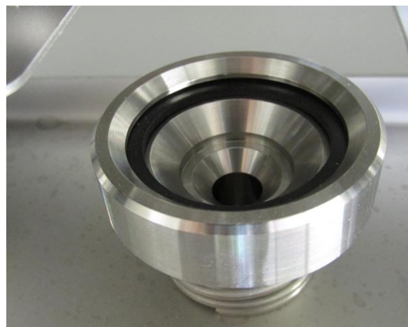
The upper flat sealing ring serves for damping, the lower one seals the connection to the crucible
