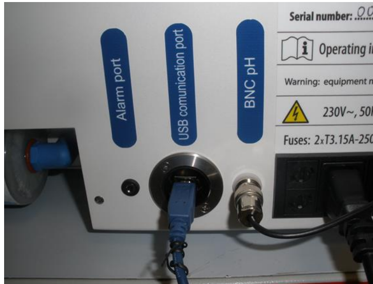
Figure 7.10 pH probe connected to the BNC
