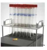
Hydroxyproline digestion thermostat, powdercoated
