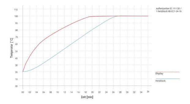
Temperature control using the example of an EC-1V metal block thermostat
