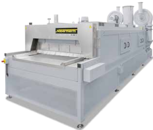
Continuous furnace D 1500/3000/300/14 for thermal ageing with mesh belt transport system and subsequent cooling station
