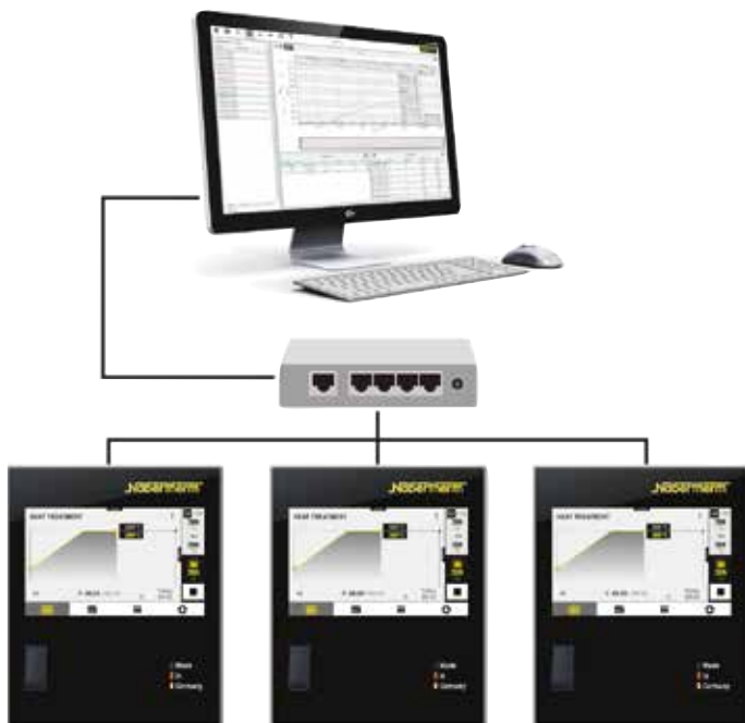
Example lay-out with 3 furnaces
