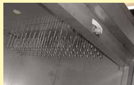
Enclosed heater coils on electrically heated models
