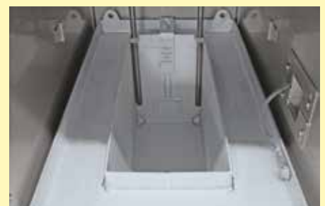
Crucible made of high-quality CrNi steel
