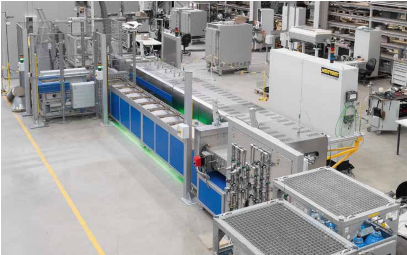
Pusher-type furnace system D 520/2600/55-04 S to sinter teflon coatings under protective atmosphere
