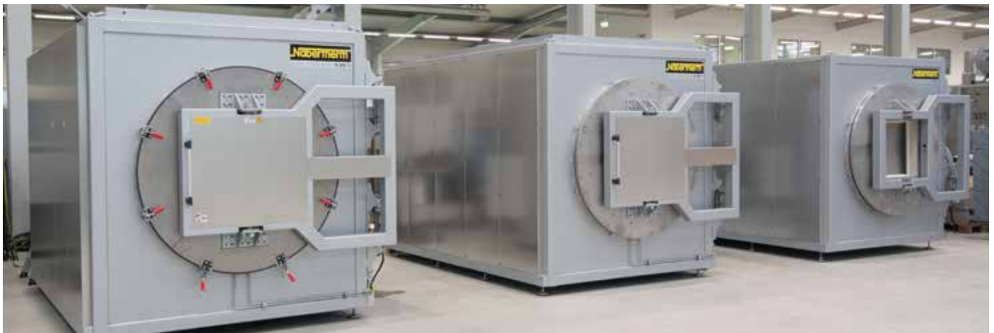
Hot-wall retort furnaces NR 1000/11 in production
