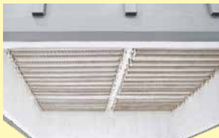
Heating elements in furnace hood
