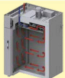
Deviation from measuring point to the average temperature in the work space e. g. \pm 3 K
