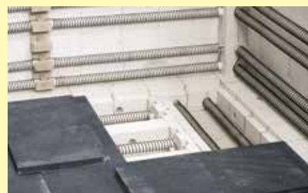
Bottom heating covered by SiC tiles to create level stacking support
