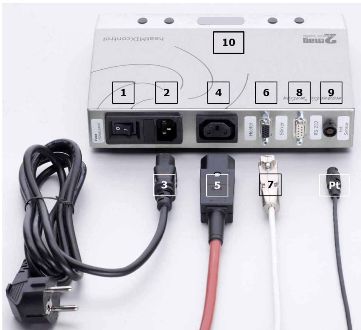
Image 4: Installation, rear side of the control unit heatMIXcontrol 230 V
